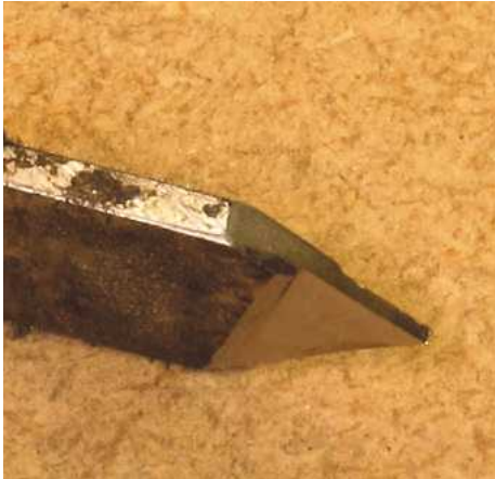
▲ Pic.19 The baize on the bottom will be sat into a groove. Les has ground an old parting tool – any old tool will do – so it has a 1mm cutting tip to cope with the small cut
